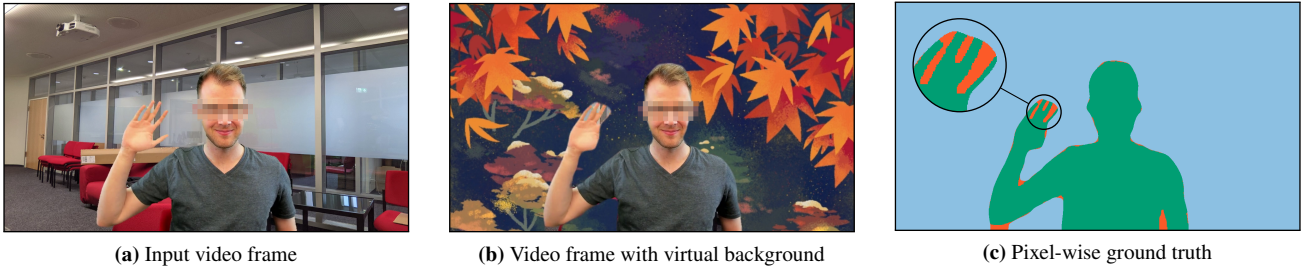
Figure 7: Example of evaluation video. (a) Video frame composed of a person and a room image. (b) Virtual background as generated by Zoom. (c) Ground truth for frame (● = environment, ● = virtual background, ● = foreground).
