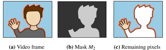
Figure 5: Partial removal of foreground using human segmentation (● = environment, ● = virtual bg). The video caller is removed using a semantic segmentation, such as DeepLabv3.
