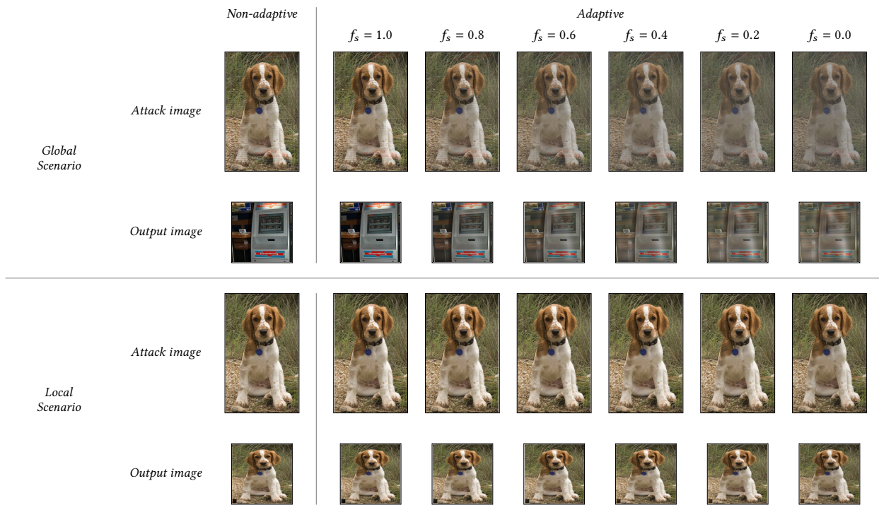
Figure 10: Evaluation examples for the adaptive attack based on suppressing peaks. The first column shows the non-adaptive, original scaling attack, while the further columns show the adaptive modification to bypass the detection. It is visible that small values of f_s have a clear impact in the global scenario.
