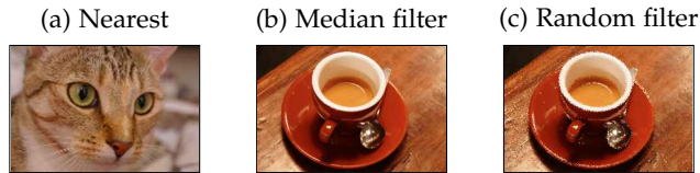
Figure 4.13: Examples of second defense: (a) insecure nearest-neighbor scaling, (b) robust scaling via selective median filter, and (c) selective random filter. Note that attack traces are not visible anymore.
